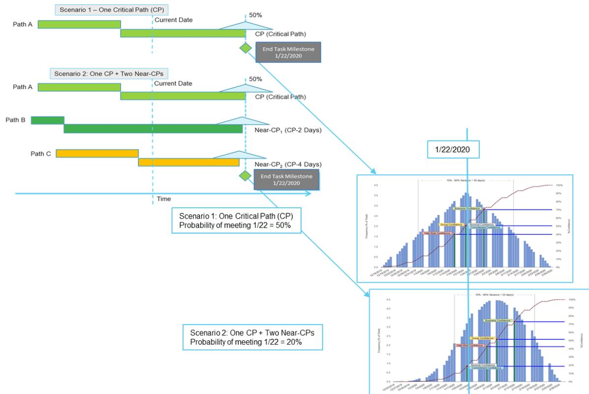
Figure 70 Simulation Results for Example “Merge Bias” Scenarios
