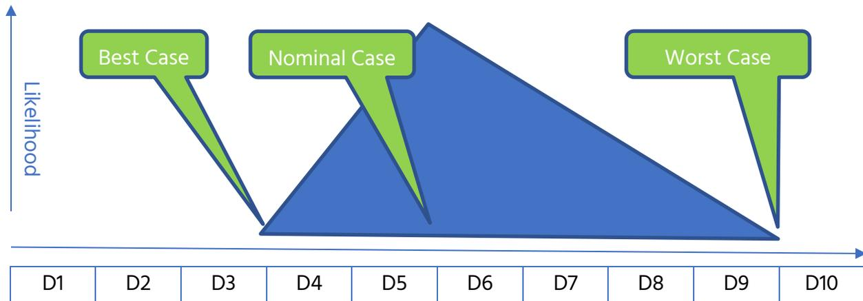
*Figure 61 3-Point Timeline Estimate for Install Plumbing*
