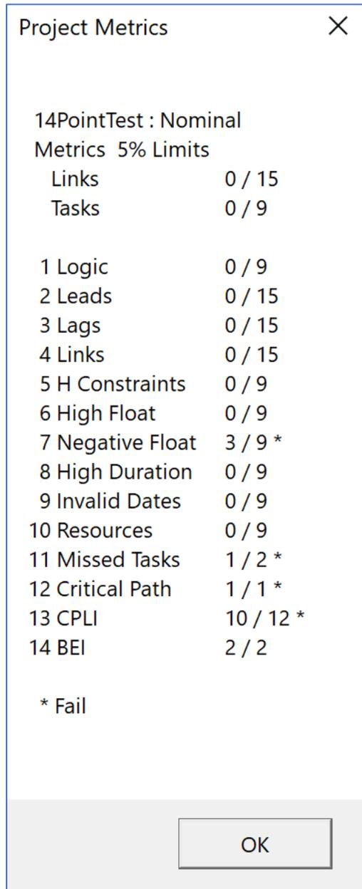
*Figure 65 Example of the DCMA 14-point Metric Scorecard Produced by Chrono™*
